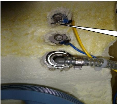
The blue & yellow wires connected to the probes in the hopper of the machine (as shown) must be tight or the system will fail.
