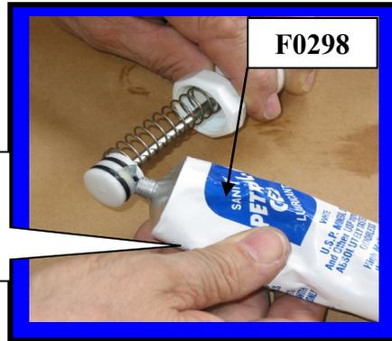
Installing **Plunger Assembly** into Faucet body
