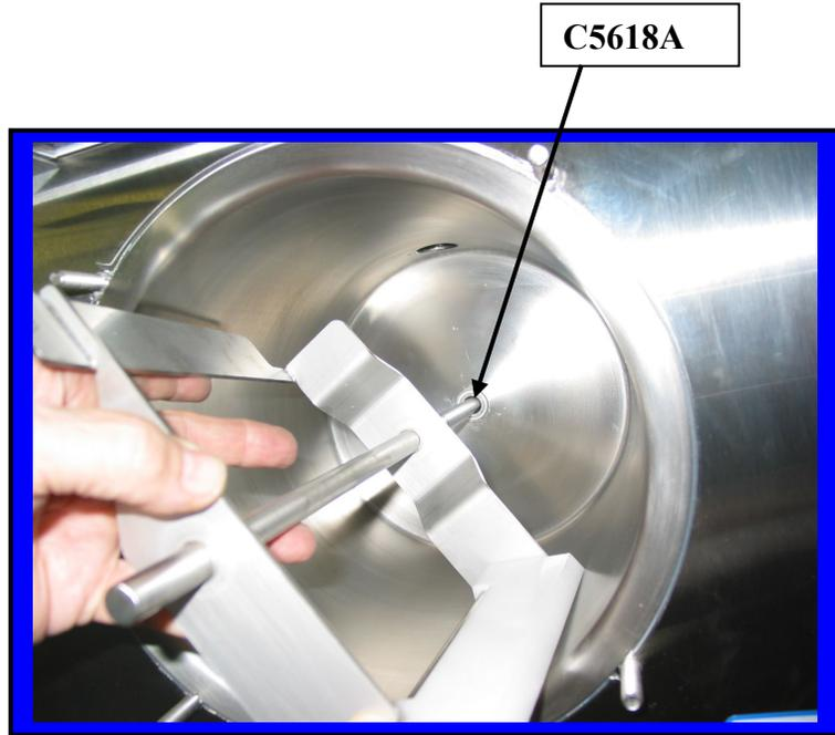
Re-install the large **faceplate** on the machine. First place the faceplate **bushing** onto the beater shaft. Then slide face plate onto the four studs. Install the faceplate knobs and tighten evenly until the faceplate O-ring is snug against the cylinder.
