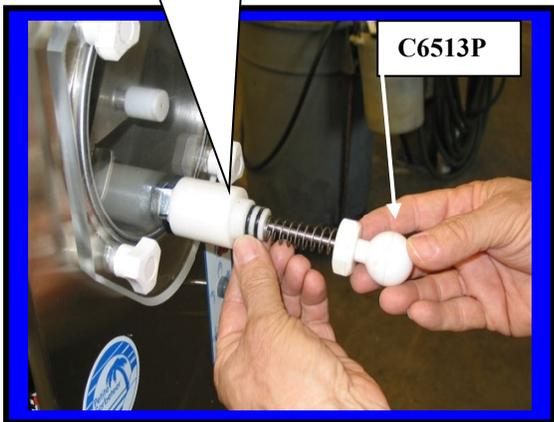
Installing large **Faceplate** onto front of Machine.
