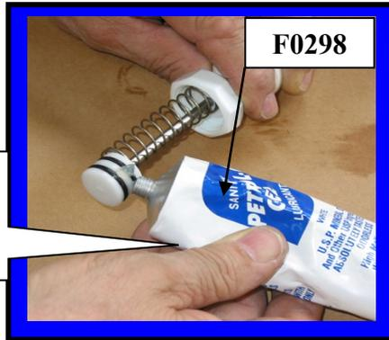
Installing **Plunger Assembly** into Faucet body
