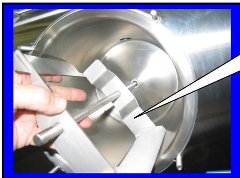
Step 7: Install beater bar assembly **C5618A** into cylinder.
