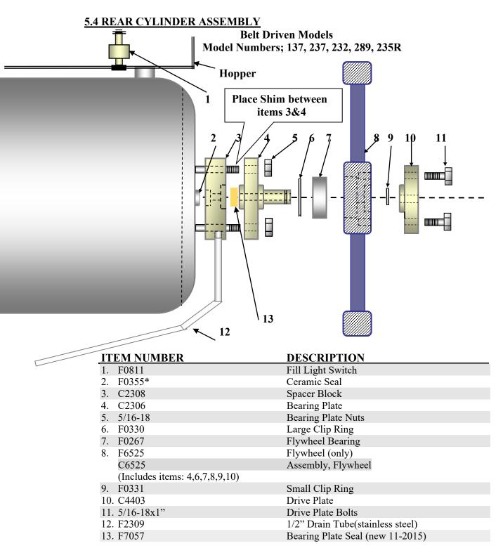
\*Note: F0355 is the part # for the Spring Seal Assembly which includes the ceramic seal. (No. 2 above)
