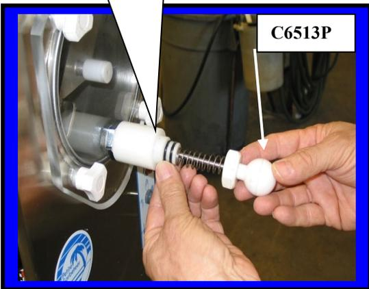
Installing large **Faceplate** onto front of Machine.
