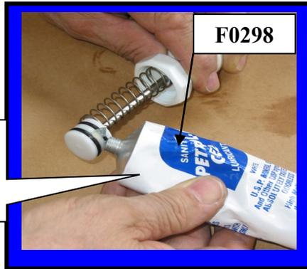
Installing **Plunger Assembly** into Faucet body
