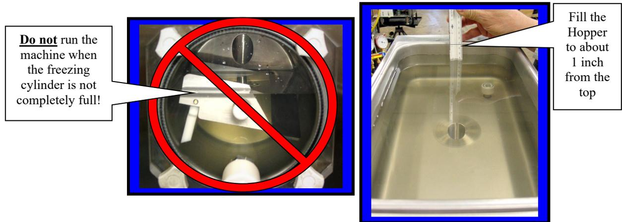
When the cylinder is full and the hopper is filled to one inch from the top, the machine is ready to run. Turn on by selecting the “right” (snowflake) position of **both** switches on the front panel.
