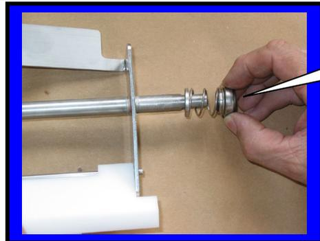
Step 5: Install spring seal F0355
