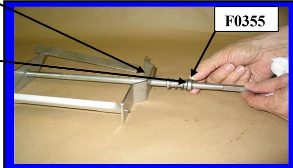
The **black carbon ring** must be facing the end of the beater bar so it will be in direct contact with the white ceramic seal inside the cylinder when the beater bar is re-installed.
