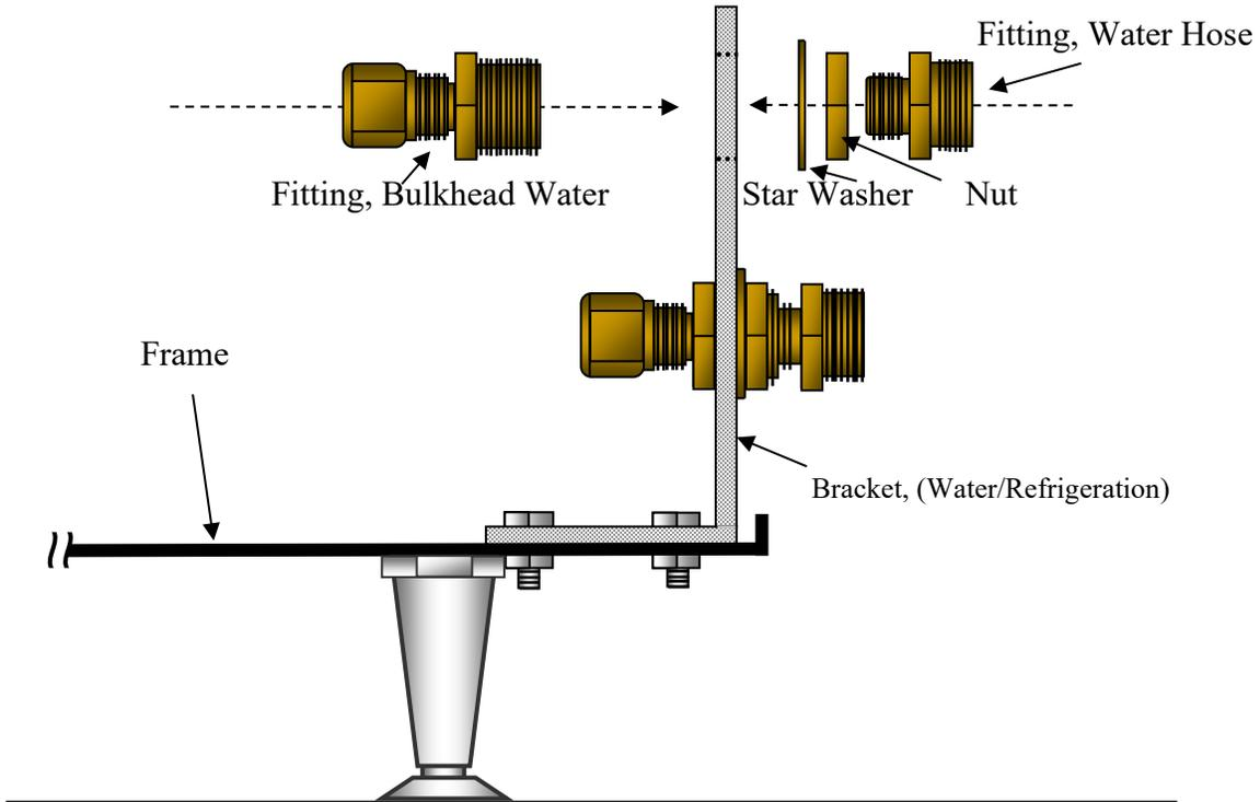
1. Insert the water bulkhead fitting through the bracket hole.
