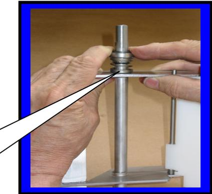
Step 6: Squeeze and release spring. Be sure the spring returns to normal before installing into machine.
