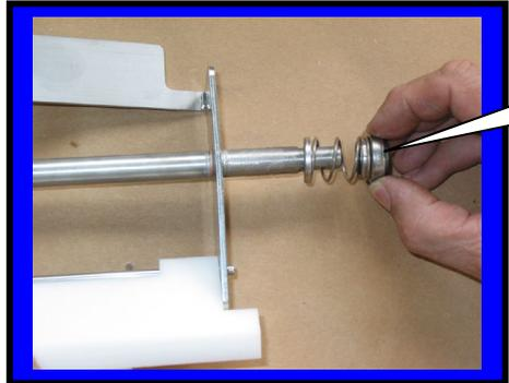
Step 5: Install spring seal F0355
