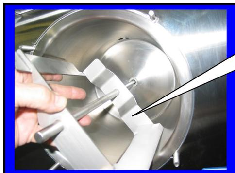
Step 7: Install large beater bar assembly C6527 into cylinder.
