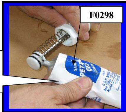
Installing **Plunger Assembly** into Faucet body
