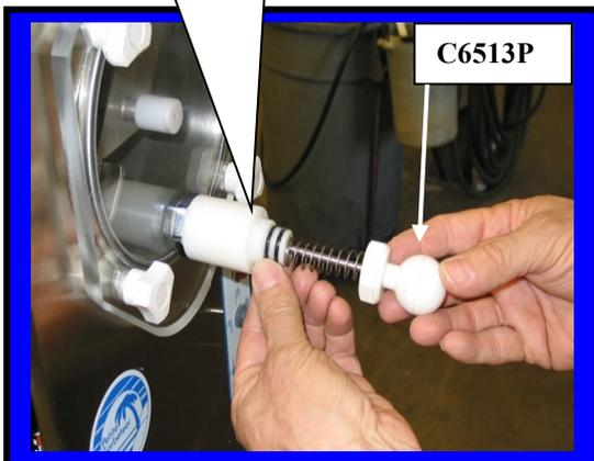
Installing large **Faceplate** onto front of Machine.
