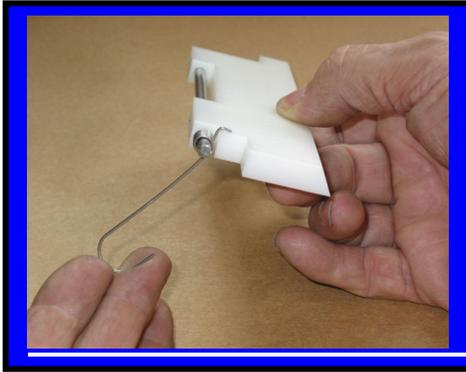
Step 1: Attach scraper blade spring F6512 as shown.
