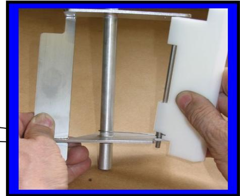
Step 2: Insert rod end into beater bar frame.
