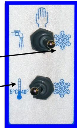
**Standby/Overnight Operation** – Top switch on **snowflake**, Bottom switch on **thermometer** symbol. Machine will automatically come on whenever necessary to keep mix cooled to 5°C/40°F - used primarily for overnight storage of mix remaining in the machine.
