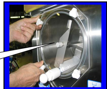
Step 8: Install large faceplate C6501 onto machine
