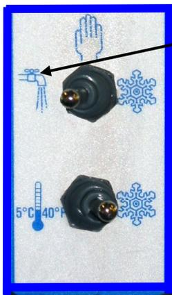
**Cleaning Operation** - The drive motor will run in the **faucet** position to allow a stirring action of the rinse water while cleaning.
