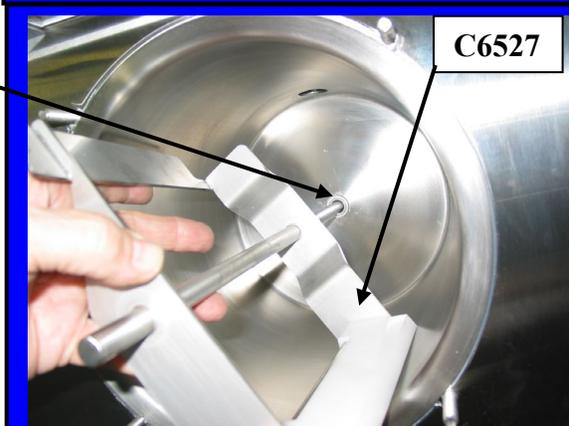
Carefully insert the large beater bar C6527 (with beater seal) into the hole at the rear of the cylinder and rotate until it fully engages into the drive plate.
