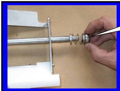
Step 5: Install spring seal F0355
