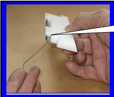
Step 1: Attach scraper blade spring F6512 as shown.
