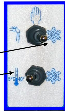
**Cooling Operation** – Top switch on **snowflake**, Bottom switch on **thermometer** symbol. Machine will automatically come on whenever necessary to keep mix cooled to 5°C/40° F - used primarily for overnight storage of mix remaining in the machine.
