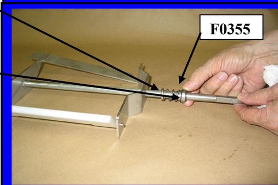
The **black carbon ring** must be facing the end of the beater bar so it will be in direct contact with the white ceramic seal inside the cylinder when the beater bar is re-installed.
