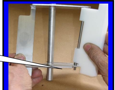
Step 2: Insert rod end into beater bar frame.
