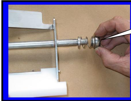
Step 5: Install spring seal F0355
