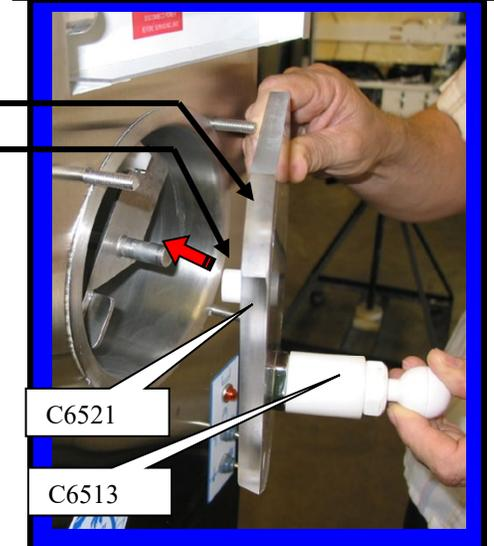
**CAUTION:** Do not over tighten the knobs or tighten against a beater bar that is not fully engaged in the drive plate; Permanent distortion to the faceplate may occur!
