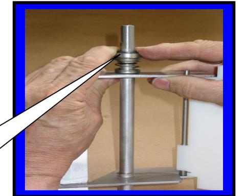
Step 6: Squeeze and release spring. Be sure the spring returns to normal before installing into machine.
