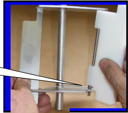
Step 2: Insert rod end into beater bar frame.
