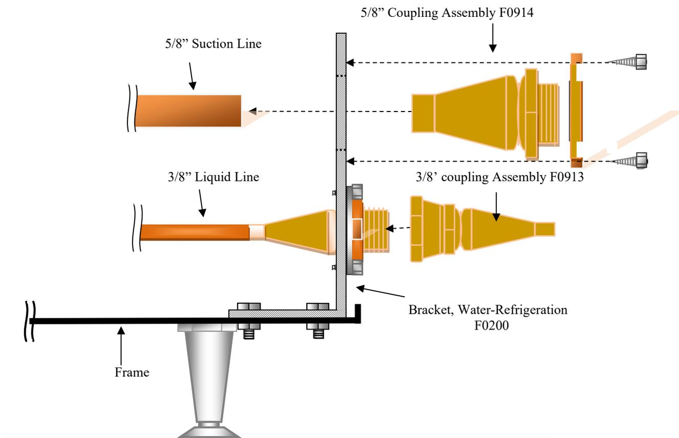
NOTE: The assemblies with part numbers F0913 and F0914 include male and female halves as well as the hold-down washer.
