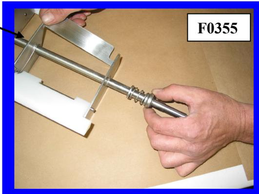
The **black carbon ring** must be facing the end of the beater bar so it will be in direct contact with the white ceramic seal inside the cylinder when the beater bar is re-installed.
