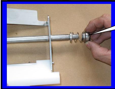
Step 5: Install spring seal F0355
