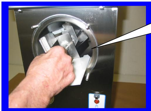
Step 7: Install beater bar assembly C6530 into cylinder.
