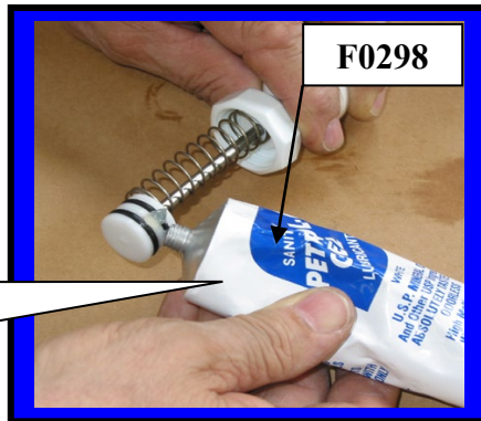
Install O-rings onto plunger
