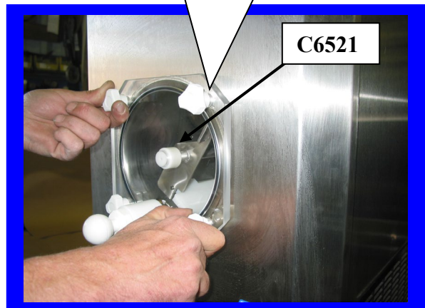
Installing small Faceplate onto front of Machine.
