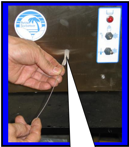
Insert long brush F6526 into drip tube
