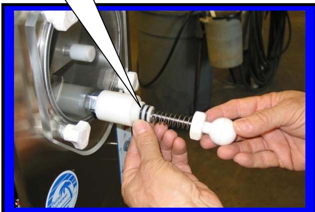
Installing Plunger assembly C6513P into faucet body
