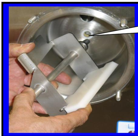
Step 7: Install beater bar C6519 into cylinder.
