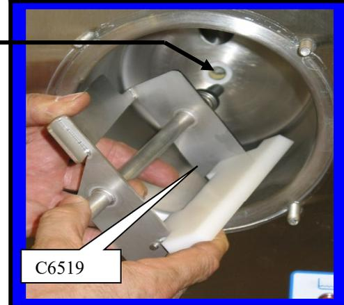
**CAUTION:** Do not strike the ceramic seal with the beater bar during installation!
