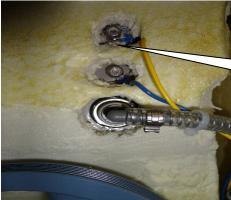
The blue & yellow wires connected to the probes in the hopper of the machine (as shown) must be tight or the system will fail.
