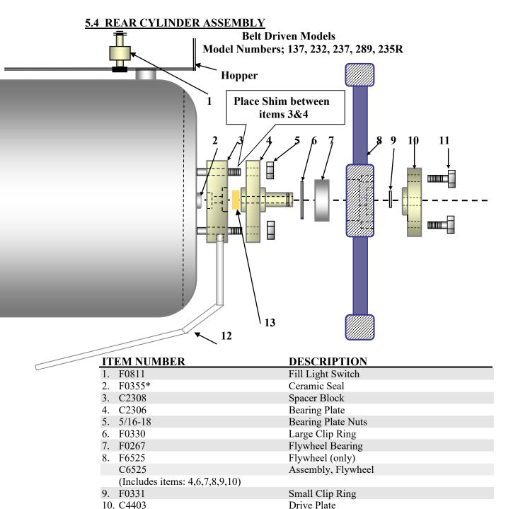
\*Note: F0355 is the part # for the Spring Seal Assembly which includes the ceramic seal. (No. 2 above)
