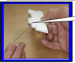
Step 1: Attach scraper blade spring **F6512** as shown.
