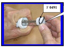
Install **O-rings** onto plunger
